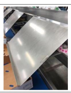
Observed that the packing tables (stainless steel) have sharp edges.
