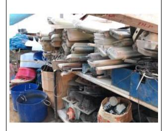
Identified lack of order and cleanliness in the workshop area (obsolete), and poor distribution of loads. Observed dangerous wastes.
